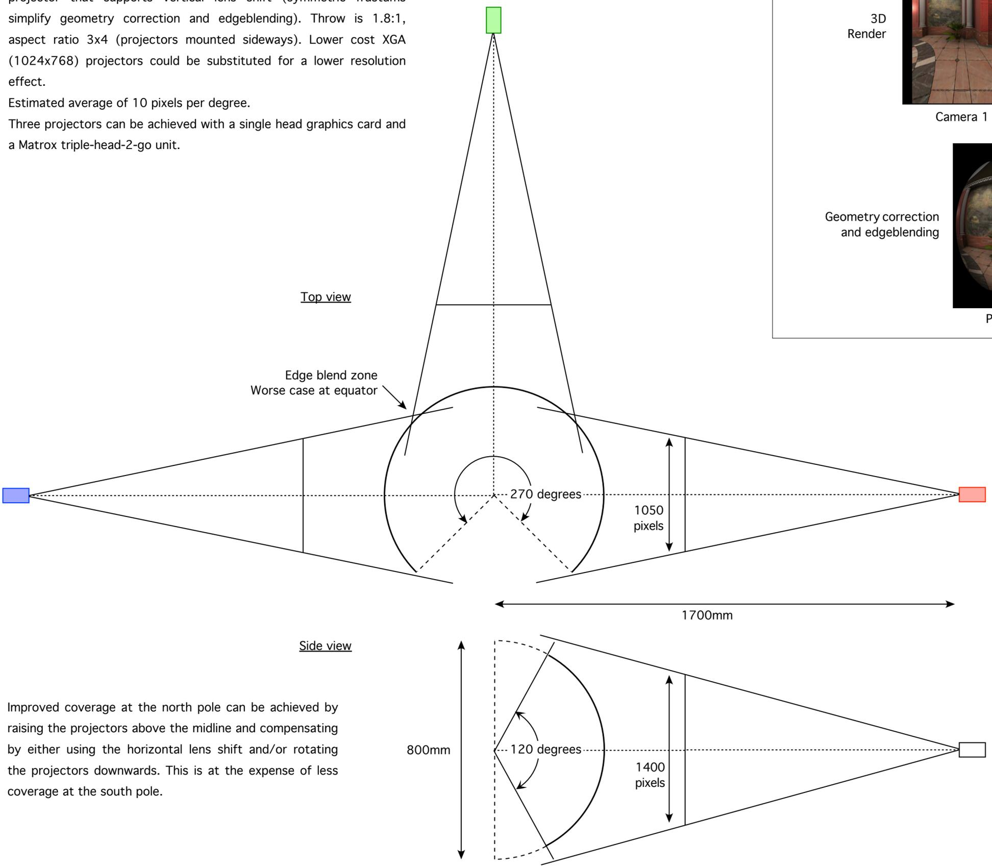
Improved coverage at the north pole can be achieved by raising the projectors above the midline and compensating by either using the horizontal lens shift and/or rotating the projectors downwards. This is at the expense of less coverage at the south pole.
