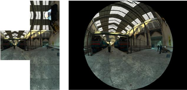
**Figure 2. Four cubic maps (left) are required to reconstruct a fisheye (right) for a hemispherical display.**
