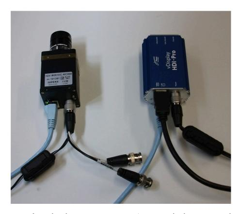
The tests were performed with a counter running at 1ms intervals, this was created as a simple Quartz Composer composition running on a low persistence display (right hand display in the photos below). The display with the counter and the display with the output from the camera are photographed together with an SLR camera using a fast shutter speed, at least 1/1000 of a second in the cases presented here.
